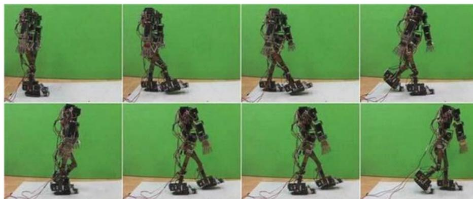
Fig. 15 A walk motion near the limit angle of heel-contact and toe-off.
